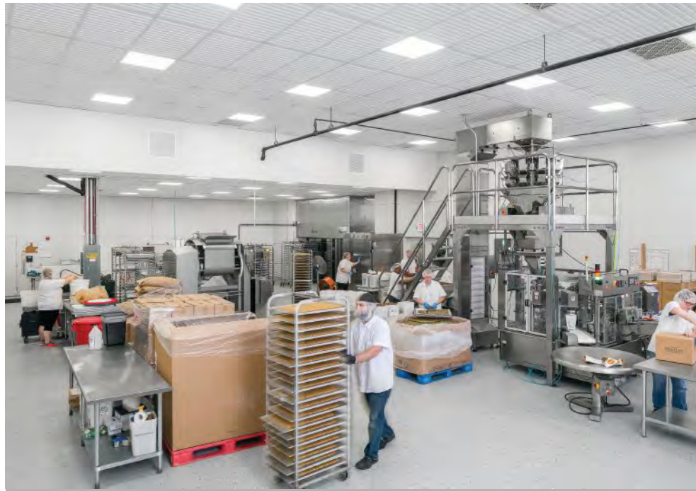
After: the refinished space is clean and bright. White ceiling panels show its cleanliness, and have good light reflectance value to help produce even illumination.
