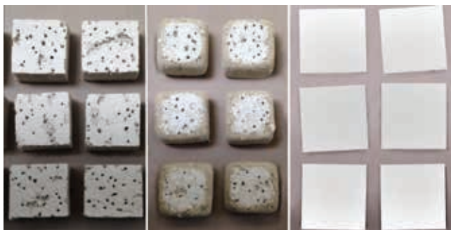
Friability test samples, (Left) mineral fiber panel specimens before testing; (Center) mineral fiber panel specimens after 20 minutes of testing; (Right) thermoformed panel specimens after 20 minutes testing (largely the same as before testing).
