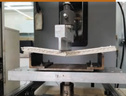
Transverse strength testing of a mineral fiber ceiling panel, a test with potential to reveal which products are more prone to breaking during handling.
