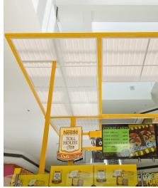
sprinklers. The panels are made of a special thermoformed material that softens at elevated temperatures. When exposed to heat from a fire, the lightweight panels drop out of a conventional ceiling grid and allow sprinklers to function properly.
