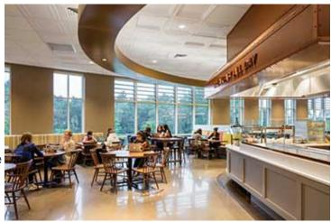
The new dining commons at Mount Holyoke College combines three styles of thermoformed ceiling panels plus mineral fiber panels to create visual scale and flow throughout the large hall. Despite the acoustically live hard surfaces and noise from the exposed kitchen, the space has good sound control, thanks in part to the noise-reducing properties of the Ceilume ceiling panels, enhanced with SonicGuard acoustic blankets above the thermoformed panels.
