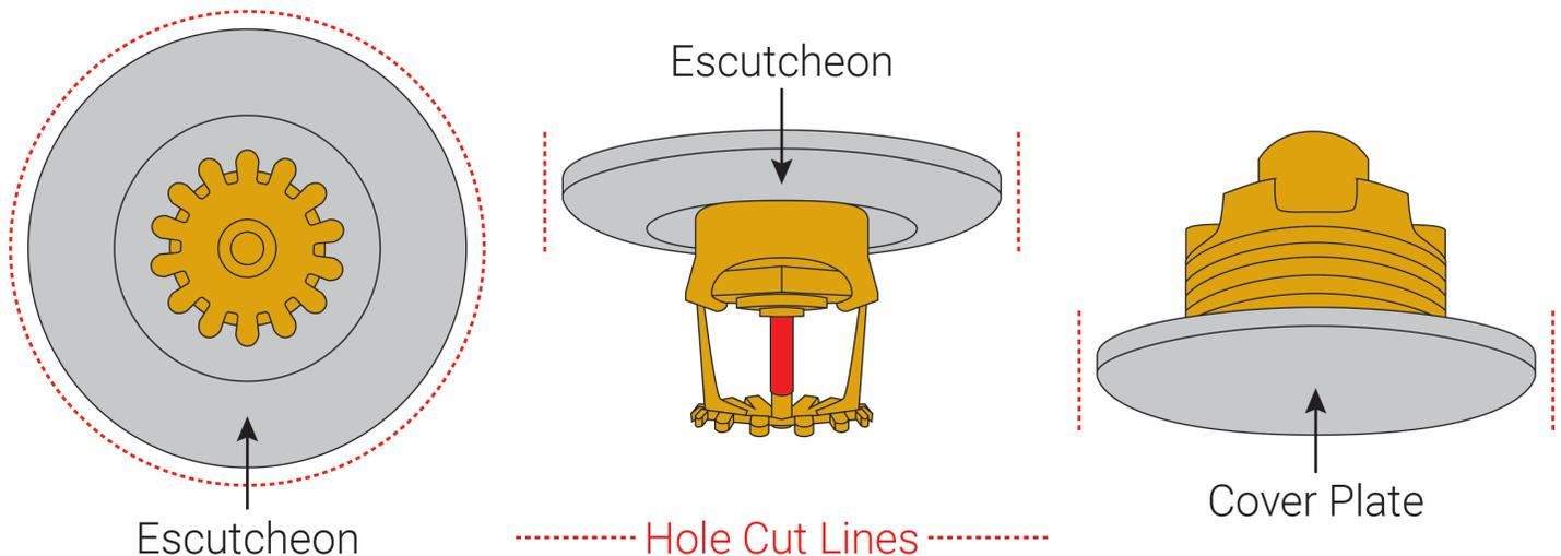
An appropriately-sized hole saw can be used to cut clean, smooth, and neat sprinkler pass-through holes. Running the saw in reverse can help keep the tile material from binding as the hole is cut.
