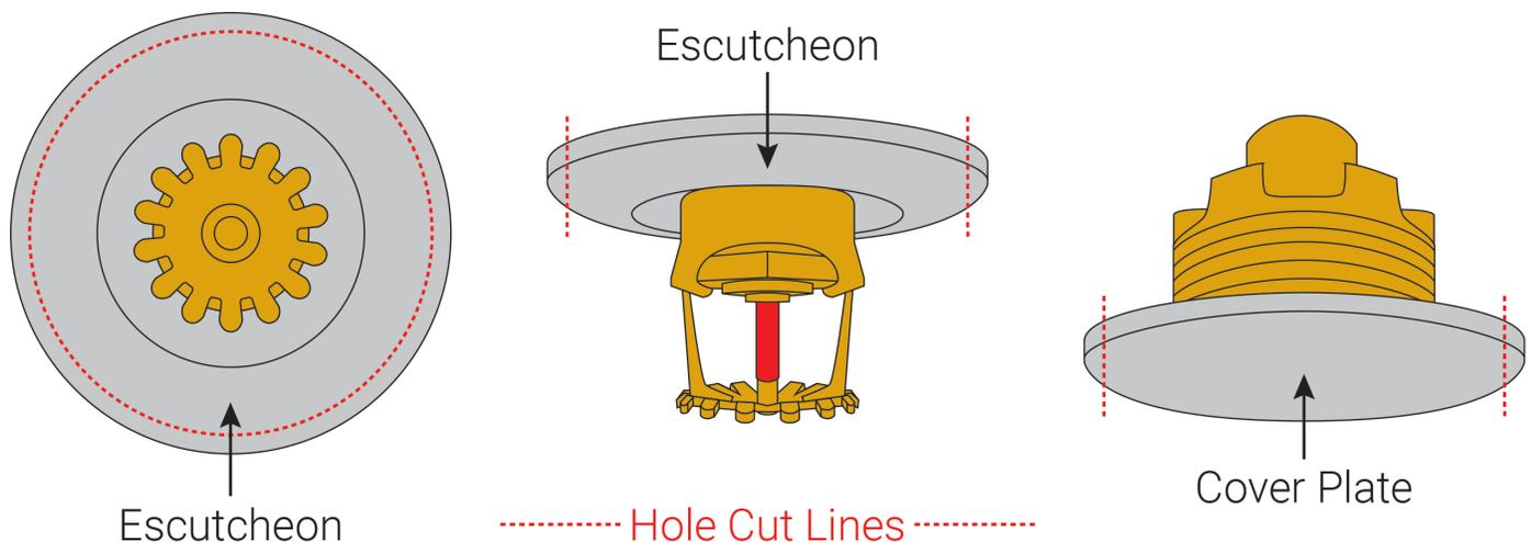
An appropriately-sized hole saw can be used to cut clean, smooth, and neat sprinkler pass-through holes in both your refacing ceiling tiles and mineral fiber backing panels. When cutting the holes in your Ceilume tiles, we suggest running the saw in reverse in order to keep the material from binding as the hole is cut.
