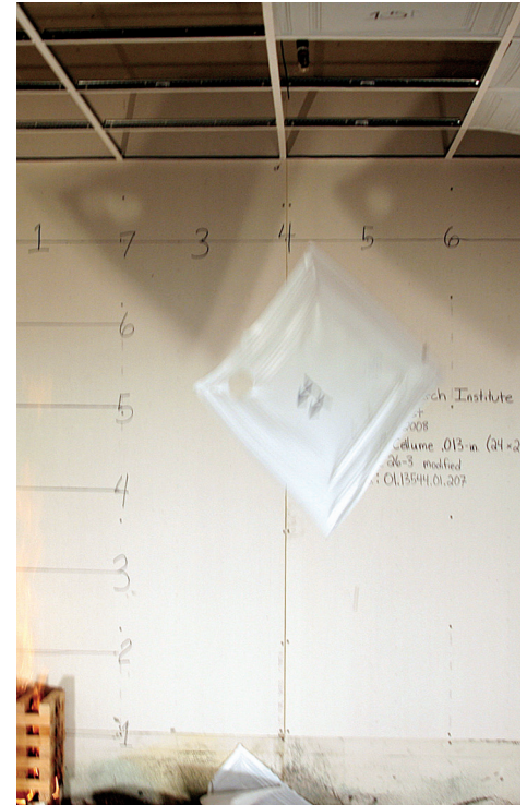
To test drop-out ceiling panels, a fire (lower left) is ignited in a corner of a room. Thermoformed panels soften when exposed to heat, deform, and drop-out of the ceiling grid before the fire grows hot enough to activate sprinklers. In this test, panels above fire have dropped-out before wood crib is fully engulfed in flame, and falling panels have not melted or ignited. The fire sprinkler, seen above falling panel, can be installed at optimal location without coordination with ceiling layout. Lab: Southwest Research Institute, San Antonio, TX / Photo: Ceilume
