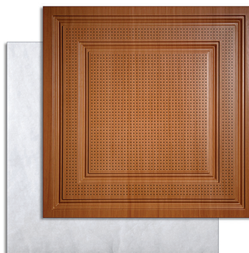
Noise reduction as high as 0.85 NRC is available with perforated thermoformed ceiling panels in combination with a thermal-bonded, polyester fiber, non-woven batt. Panels and batts are Class A rated for surface burning characteristics and panels are Greenguard Gold certified for low VOC emissions. The faux wood finish shown here provides verisimilitude when viewed at normal ceiling heights. Photo: Ceilume
