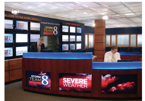
Luminous, back-lit ceiling panels create uniform illumination without the hot-spot of troffers or downlights. Sprinklers can be concealed above ceiling panels to avoid shadows that would be cast by penetrating sprinklers. The Storm Team 8 Newsroom, Grand Rapids, MI was designed by FX Design Group. Photo: WOOD-TV
