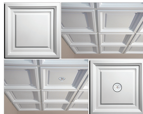
The best looking fire sprinkler, in the opinion of many designers, is the one that isn't there. Sprinklers can be installed above approved thermoformed ceilings (top) or no more than 1 inch (24 mm) beneath surface (bottom). Holes for penetrating sprinklers must be slightly oversized to allow panels to drop-out without draping over sprinklers in the event of a fire. Photo: Ceilume
