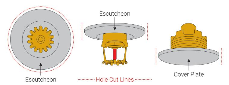
An appropriately-sized hole saw can be used to cut clean, smooth, and neat sprinkler pass-through holes. Running the saw in reverse can help keep the tile material from binding as the hole is cut.
