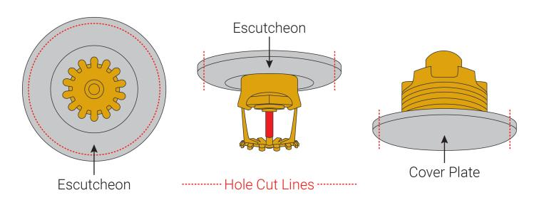
An appropriately-sized hole saw can be used to cut clean, smooth, and neat sprinkler pass-through holes in both your refacing ceiling tiles and mineral fiber backing panels. When cutting the holes in your Ceilume tiles, we suggest running the saw in reverse in order to keep the material from binding as the hole is cut.
