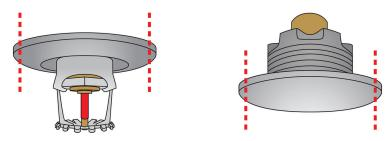
An appropriately-sized hole saw can be used to cut sprinkler-penetration holes through both mineral fiber backing panels and Ceilume tiles. When cutting the holes in your Ceilume tiles, run the saw in reverse in order to prevent tile material from binding.
