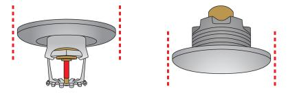
An appropriately-sized hole saw can be used to cut clean, smooth, and neat sprinkler-penetration holes. Run the saw in reverse in order to keep tile material from binding.
