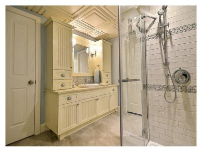
Because thermoformed ceiling tile are impervious to moisture, they are an excellent choice for wet environments like bathrooms.
