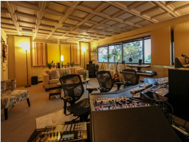
Acoustics are critical in a recording studio. A Noise Reduction Coefficient of at least NRC = 0.50 was needed to fine tune the room, and was achieved with Ceilume panels topped with Soniguard itch-free polyester batt insulation.
