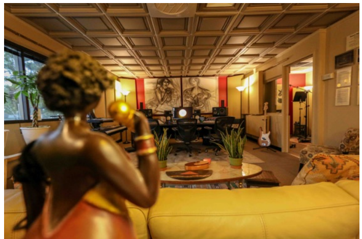
Acoustics are critical in a recording studio. A Noise Reduction Coefficient of at least NRC = 0.50 was needed to fine tune the room, and was achieved with Ceilume panels topped with Soniguard itch-free polyester batt insulation.
