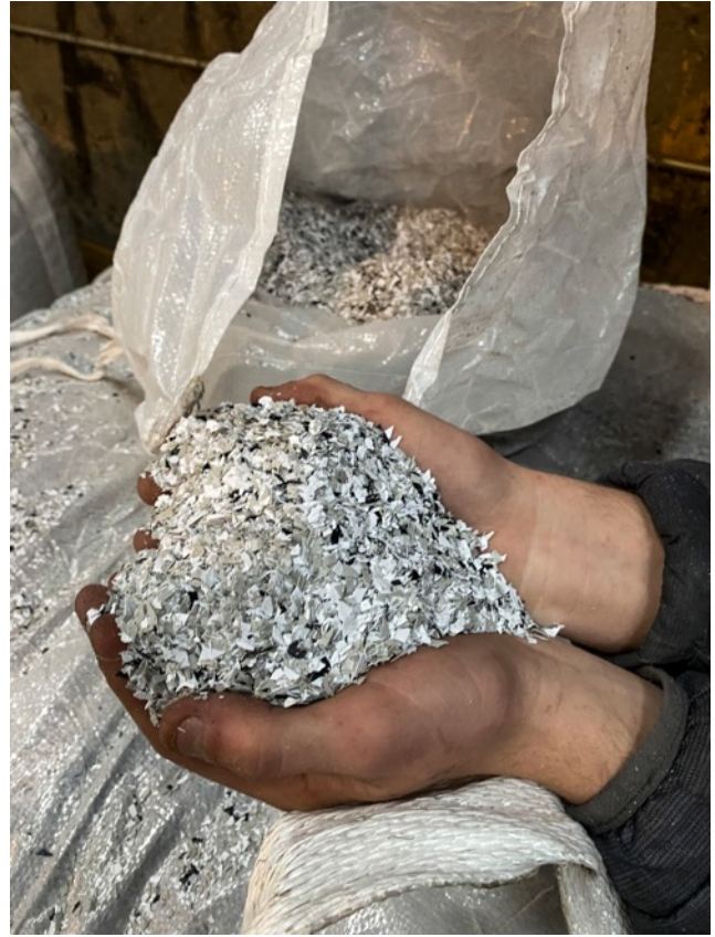
Used panels are collected from customers after their service life is over ( left ) and mixed with the limited amount of waste produced by Ceilume's thermoforming process. They are chipped ( right ) for recycling.
